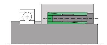
Using SIT-LOCK® 15 to lock a hub while axially locking a bearing. For further information, please contact our Technical Department.
